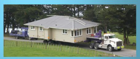
The use of transportable classrooms means that new schools can be developed, additional capacity added, and emergency classrooms made available at short notice.
